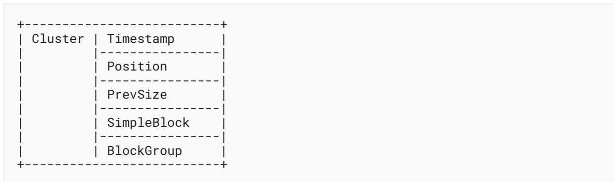
Figure 6: Representation of a Cluster Element and Its Immediate Child Elements
