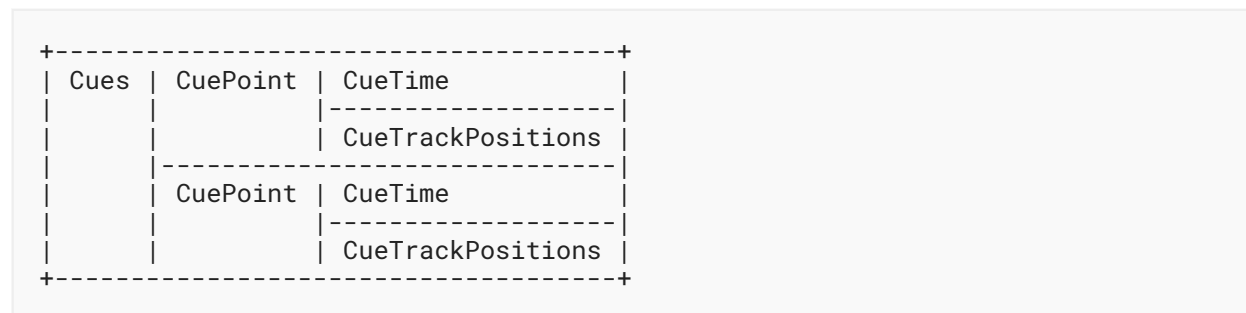
Figure 8: Representation of a Cues Element and Two Levels of Its Descendant Elements
