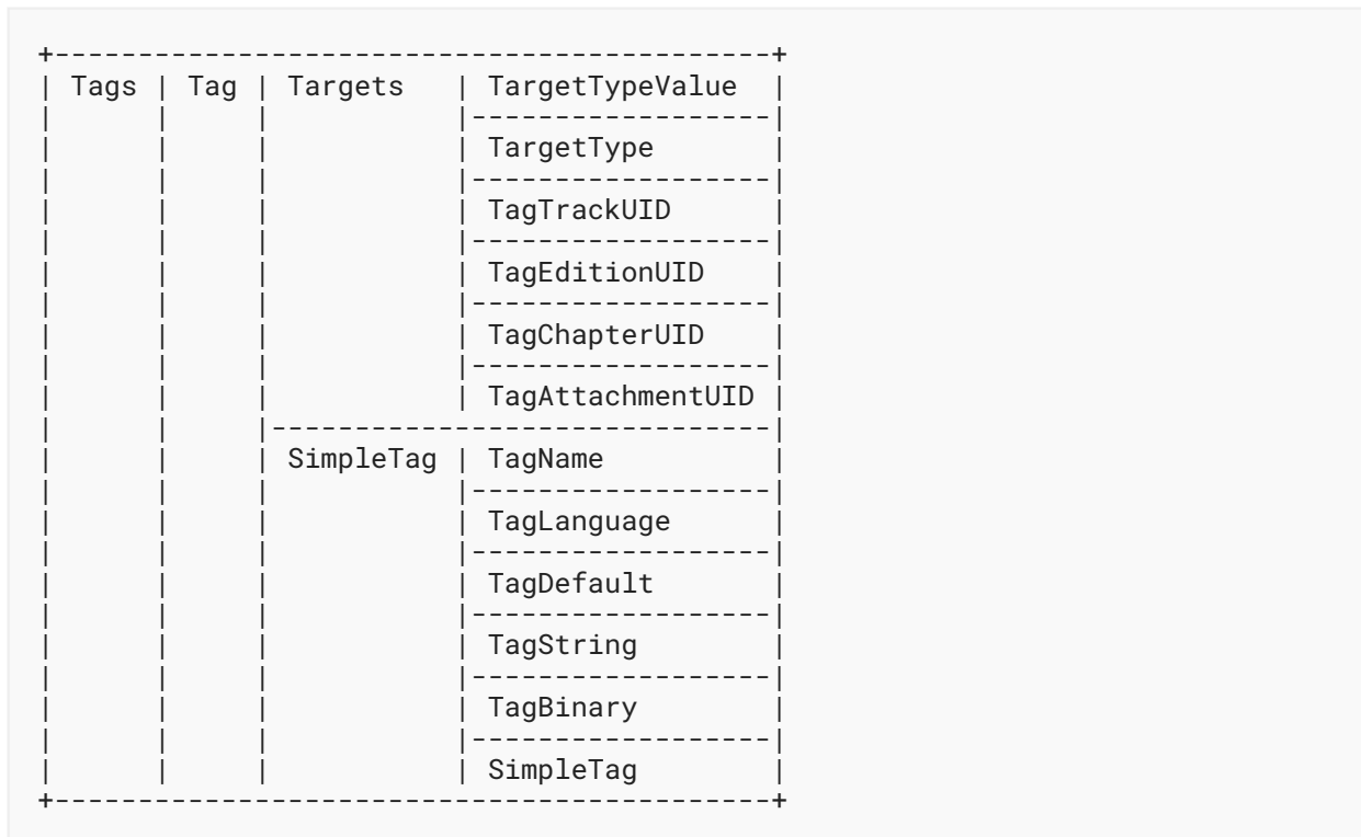
Figure 10: Representation of a Tags Element and Three Levels of Its Children Elements
