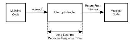
Figure 14.12: Non-Threaded Interrupt Handler
