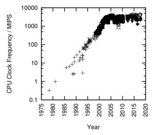
Figure 2.1: MIPS/Clock-Frequency Trend for Intel CPUs
