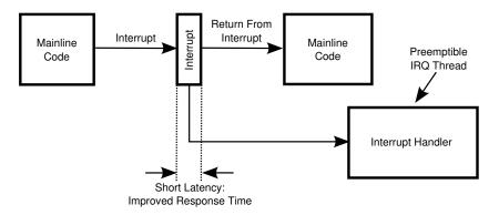
Figure 14.13: Threaded Interrupt Handler
