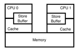
Figure 15.1: System Architecture With Store Buffers
