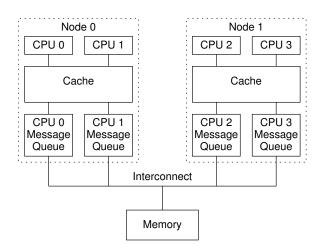
Figure C.8: Example Ordering-Hostile Architecture
