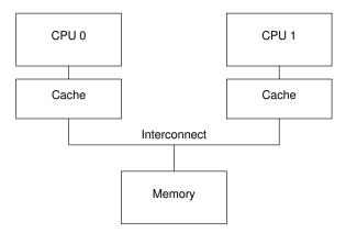
Figure C.1: Modern Computer System Cache Structure
