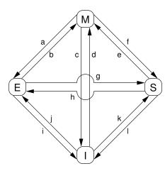
Figure C.3: MESI Cache-Coherency State Diagram
