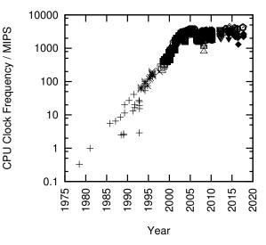
Figure 6.11: MIPS/Clock-Frequency Trend for Intel CPUs
