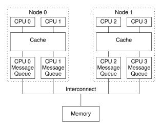
Figure C.8: Example Ordering-Hostile Architecture
