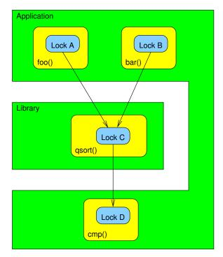
Figure 7.6: Layered Locking Hierarchy for qsort()
