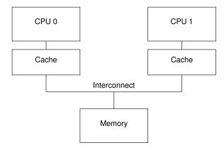
Figure C.1: Modern Computer System Cache Structure
