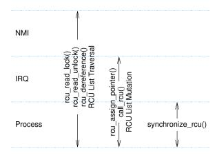
Figure 9.20: RCU API Usage Constraints
