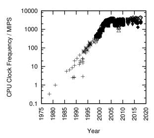
**Figure 6.11:** MIPS/Clock-Frequency Trend for Intel CPUs
