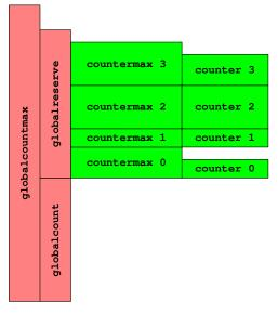
Figure 5.5: Simple Limit Counter Variable Relationships
