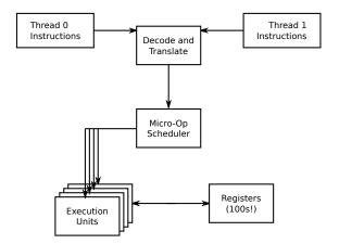
Figure 3.4: Rough View of Modern Micro-Architecture
