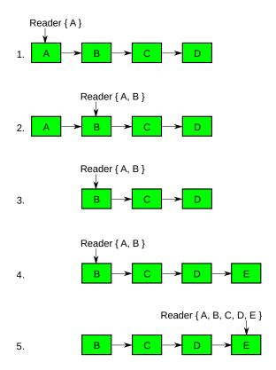
Figure 9.15: Multiple RCU Data-Structure Versions
