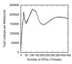
**Figure 10.4:** Read-Only Hash-Table Performance For Schrödinger's Zoo, Varying Buckets
