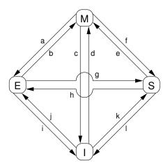
Figure C.3: MESI Cache-Coherency State Diagram
