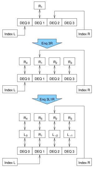
Figure 6.8: Hashed Double-Ended Queue After Insertions
