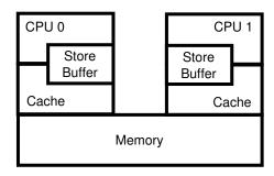
Figure 15.1: System Architecture With Store Buffers
