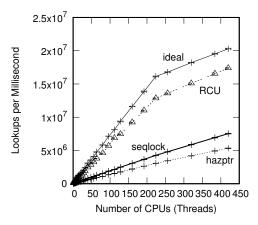
Figure 9.21: Pre-BSD Routing Table Protected by RCU
