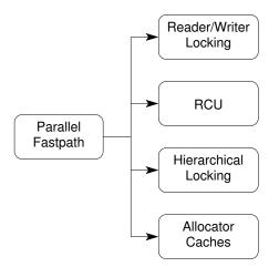
Figure 6.18: Parallel-Fastpath Design Patterns
