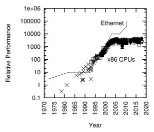
**Figure 6.12:** Ethernet Bandwidth vs. Intel x86 CPU Performance
