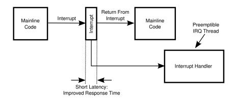
Figure 14.13: Threaded Interrupt Handler
