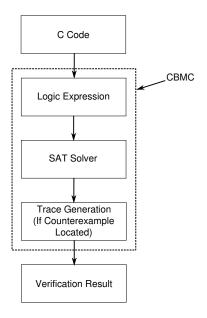
Figure 12.2: CBMC Processing Flow
