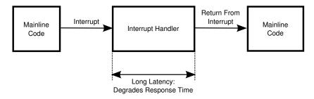
Figure 14.12: Non-Threaded Interrupt Handler
