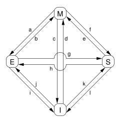
Figure C.3: MESI Cache-Coherency State Diagram
