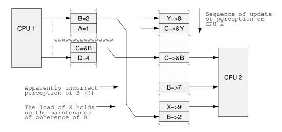
Figure 12.8: Data Dependency Barrier Omitted
