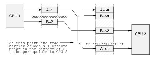
Figure 12.11: Read Barrier Supplied
