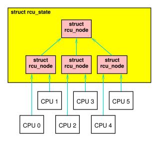
Figure D.12: Hierarchical RCU State
