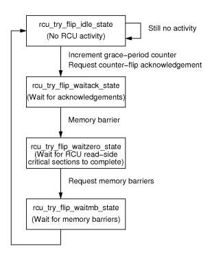
Figure D.63: Preemptible RCU State Machine
