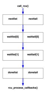
Figure D.62: Preemptible RCU Callback Flow
