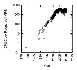
Figure 1.1: MIPS/Clock-Frequency Trend for Intel CPUs
