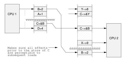
Figure 12.9: Data Dependency Barrier Supplied
