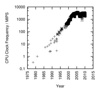
Figure 5.14: MIPS/Clock-Frequency Trend for Intel CPUs
