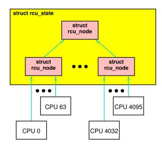
Figure D.15: Hierarchical RCU State 4,096 CPUs
