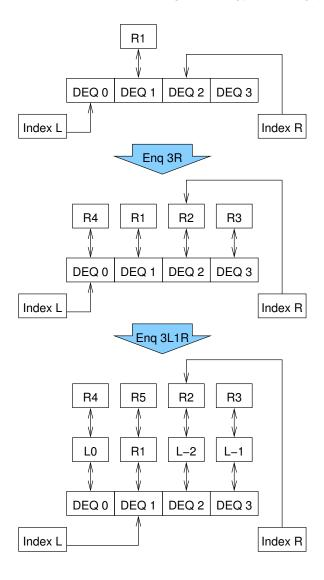
Figure 5.8: Hashed Double-Ended Queue After Insertions
