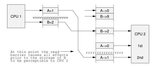
Figure 12.12: Read Barrier Supplied, Double Load
