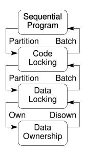
Figure 5.13: Design Patterns and Lock Granularity
