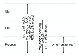
Figure 8.33: RCU API Usage Constraints
