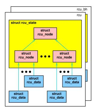
Figure D.16: Hierarchical RCU State With BH
