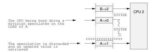
Figure 12.16: Speculative Load Cancelled by Barrier
