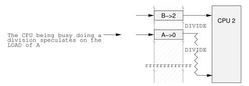
Figure 12.15: Speculative Load and Barrier
