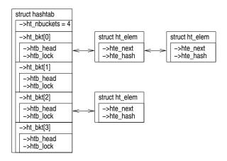
Figure 11.2: Hash-Table Data-Structure Diagram
