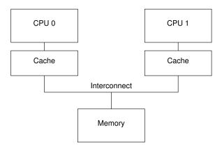
Figure 12.1: Modern Computer System Cache Structure
