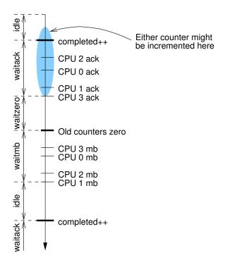
Figure D.64: Preemptible RCU State Machine Timeline
