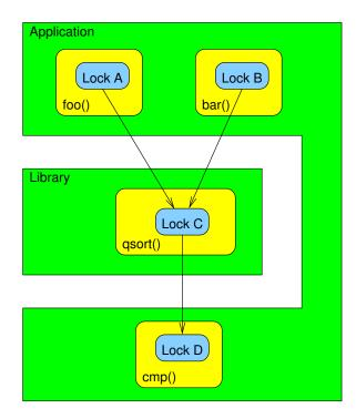
Figure 6.6: Layered Locking Hierarchy for qsort()
