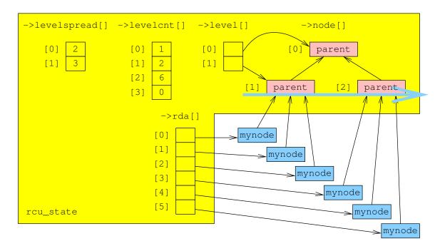
Figure D.52: Scanning Leaf rcu\_node Structures
