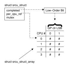
Figure D.5: SRCU Data-Structure Diagram
