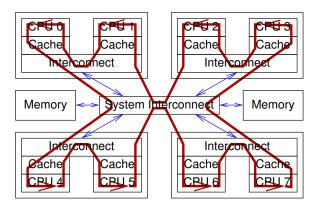
Figure 4.4: Data Flow For Global Atomic Increment
