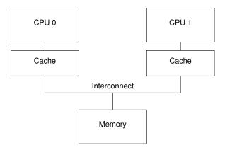
Figure C.1: Modern Computer System Cache Structure
