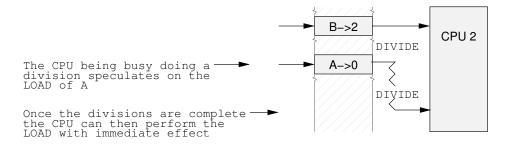
Figure 12.14: Speculative Load
