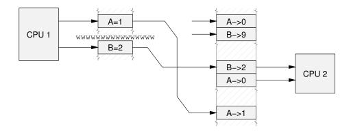
Figure 12.10: Read Barrier Needed
