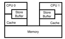
Figure 15.1: System Architecture With Store Buffers
