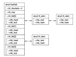
Figure 10.1: Hash-Table Data-Structure Diagram
