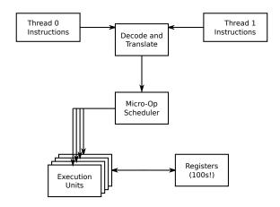
Figure 3.4: Rough View of Modern Micro-Architecture
