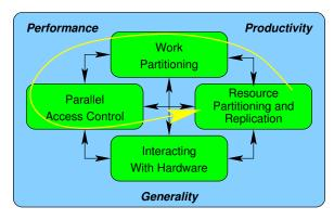
Figure 2.6: Ordering of Parallel-Programming Tasks
