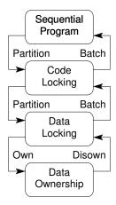
Figure 6.10: Design Patterns and Lock Granularity
