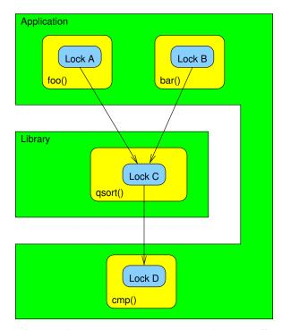
Figure 7.6: Layered Locking Hierarchy for qsort()
