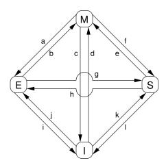
Figure C.3: MESI Cache-Coherency State Diagram
