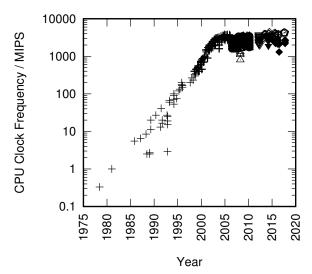
Figure 2.1: MIPS/Clock-Frequency Trend for Intel CPUs
