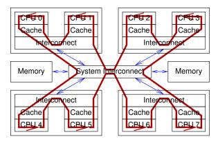
Figure 5.2: Data Flow For Global Atomic Increment
