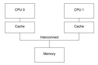
Figure C.1: Modern Computer System Cache Structure
