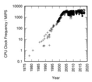
Figure 6.11: MIPS/Clock-Frequency Trend for Intel CPUs
