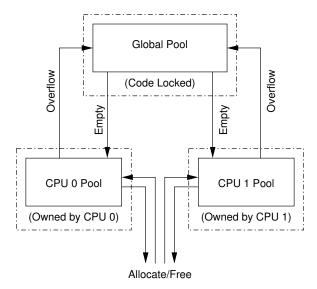
Figure 6.19: Allocator Cache Schematic
