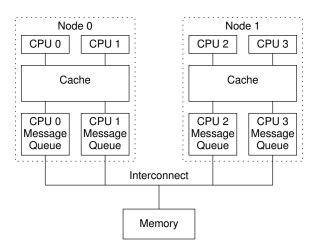
Figure C.8: Example Ordering-Hostile Architecture
