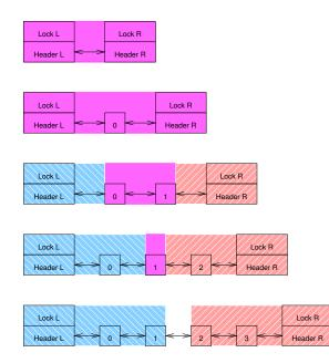
Figure 6.5: Double-Ended Queue With Left- and Right-Hand Locks
