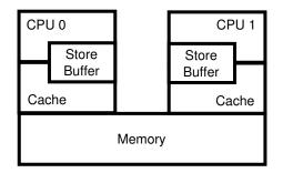
Figure 15.1: System Architecture With Store Buffers
