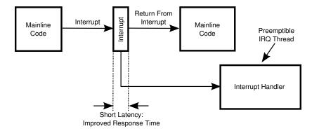
Figure 14.13: Threaded Interrupt Handler
