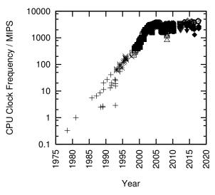
Figure 2.1: MIPS/Clock-Frequency Trend for Intel CPUs
