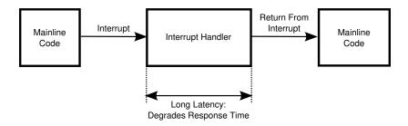
Figure 14.12: Non-Threaded Interrupt Handler
