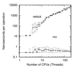
Figure 9.23: Performance Advantage of RCU Over Reader-Writer Locking
