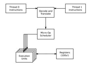
Figure 3.4: Rough View of Modern Micro-Architecture
