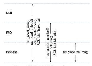
Figure 9.20: RCU API Usage Constraints
