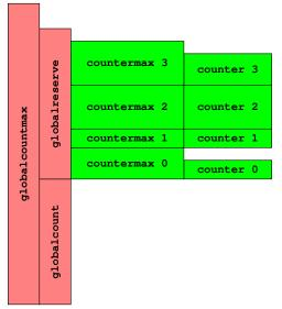
Figure 5.5: Simple Limit Counter Variable Relationships
