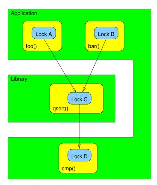
Figure 7.6: Layered Locking Hierarchy for qsort()
