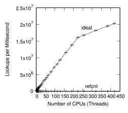
Figure 9.2: Pre-BSD Routing Table Protected by Reference Counting
