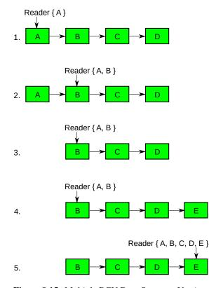
Figure 9.15: Multiple RCU Data-Structure Versions
