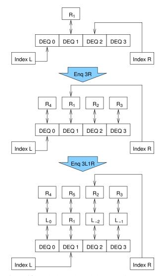
Figure 6.8: Hashed Double-Ended Queue After Insertions
