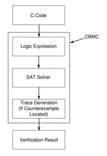
Figure 12.2: CBMC Processing Flow
