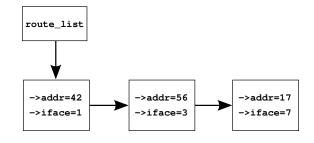
Figure 9.1: Pre-BSD Packet Routing List
