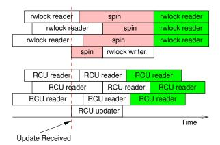
Figure 9.26: Response Time of RCU vs. Reader-Writer Locking
