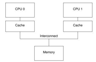
Figure C.1: Modern Computer System Cache Structure
