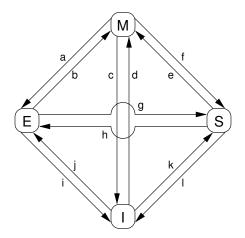
Figure C.3: MESI Cache-Coherency State Diagram
