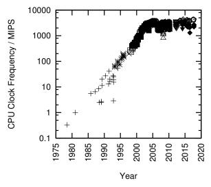
Figure 6.11: MIPS/Clock-Frequency Trend for Intel CPUs
